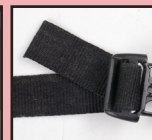
Webbing termination cut off
