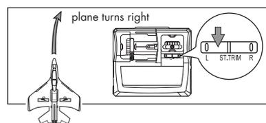
4. Push the direction stick toward left to turn the plane anticlockwise, and push the direction stick toward right to turn it clockwise. The plane turns depending on the speed difference between the left propellers and the right propellers.
