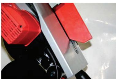
Lift the saw. Remove the plastic fuse at the base of the saw. Save fuse. He will have to put back into place when you want to use the machine as circular saw with board.
