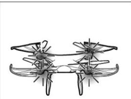
When the battery is low, the drone's 4 LEDs start to flash. The drone lands automatically.
