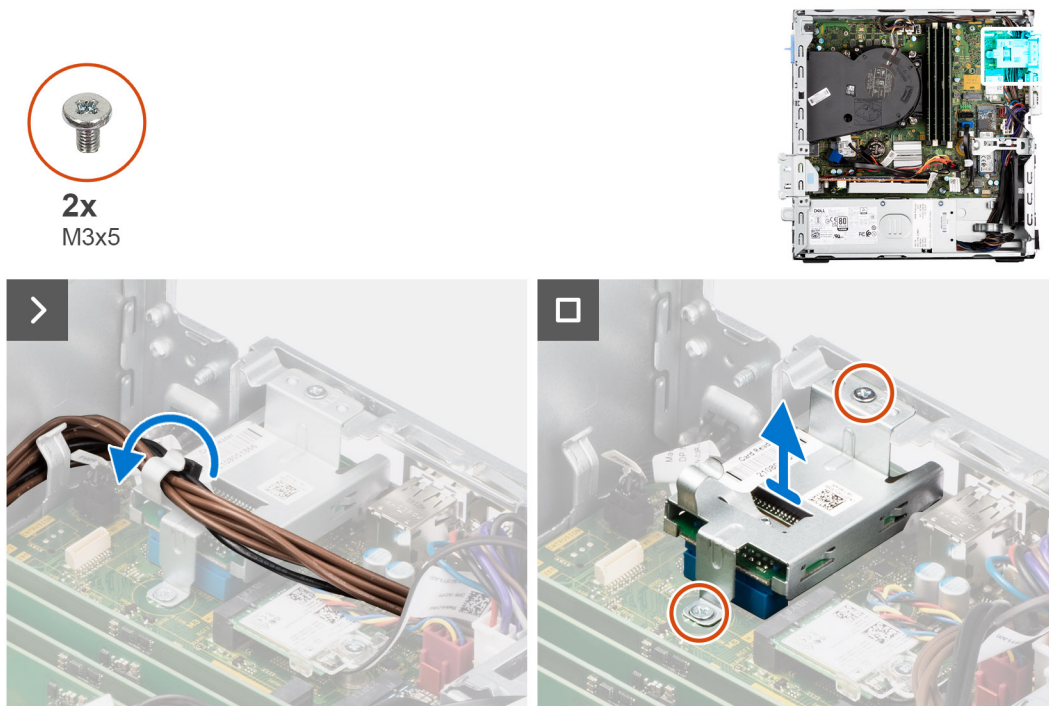
Figure 31. Removing the media-card reader
