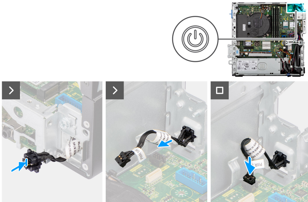
Figure 40. Installing the power button
