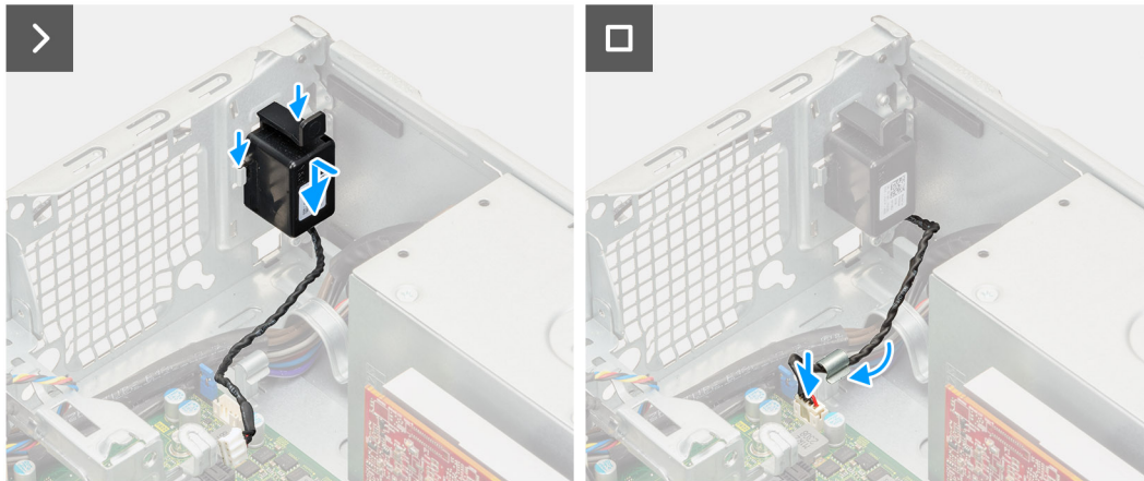
Figure 36. Installing the speaker
