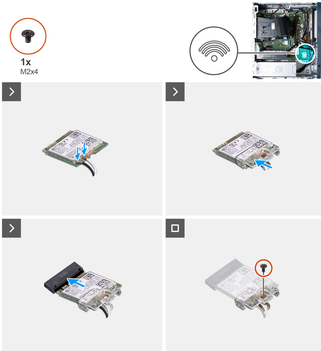
Figure 21. Installing the wireless card
