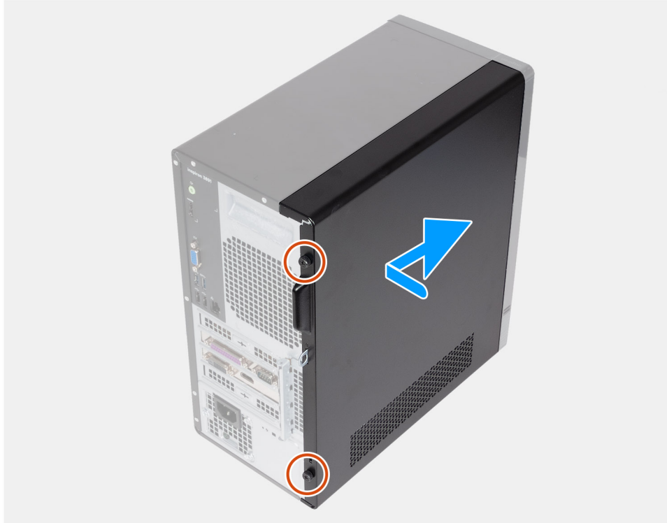
Figure 11. Installing the left-side cover
