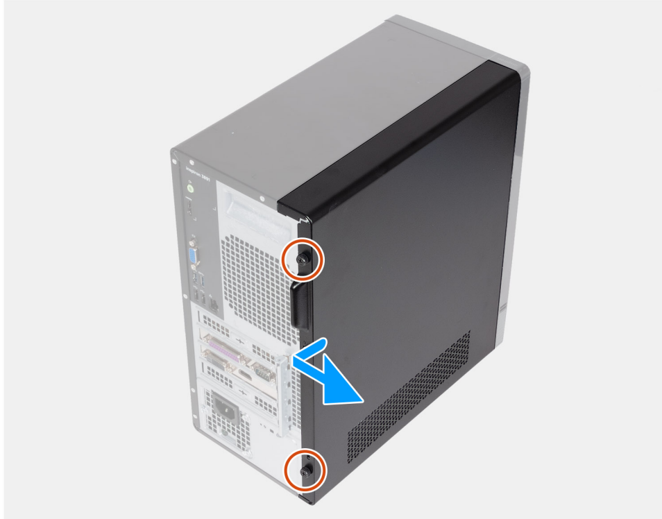
Figure 10. Removing the left-side cover
