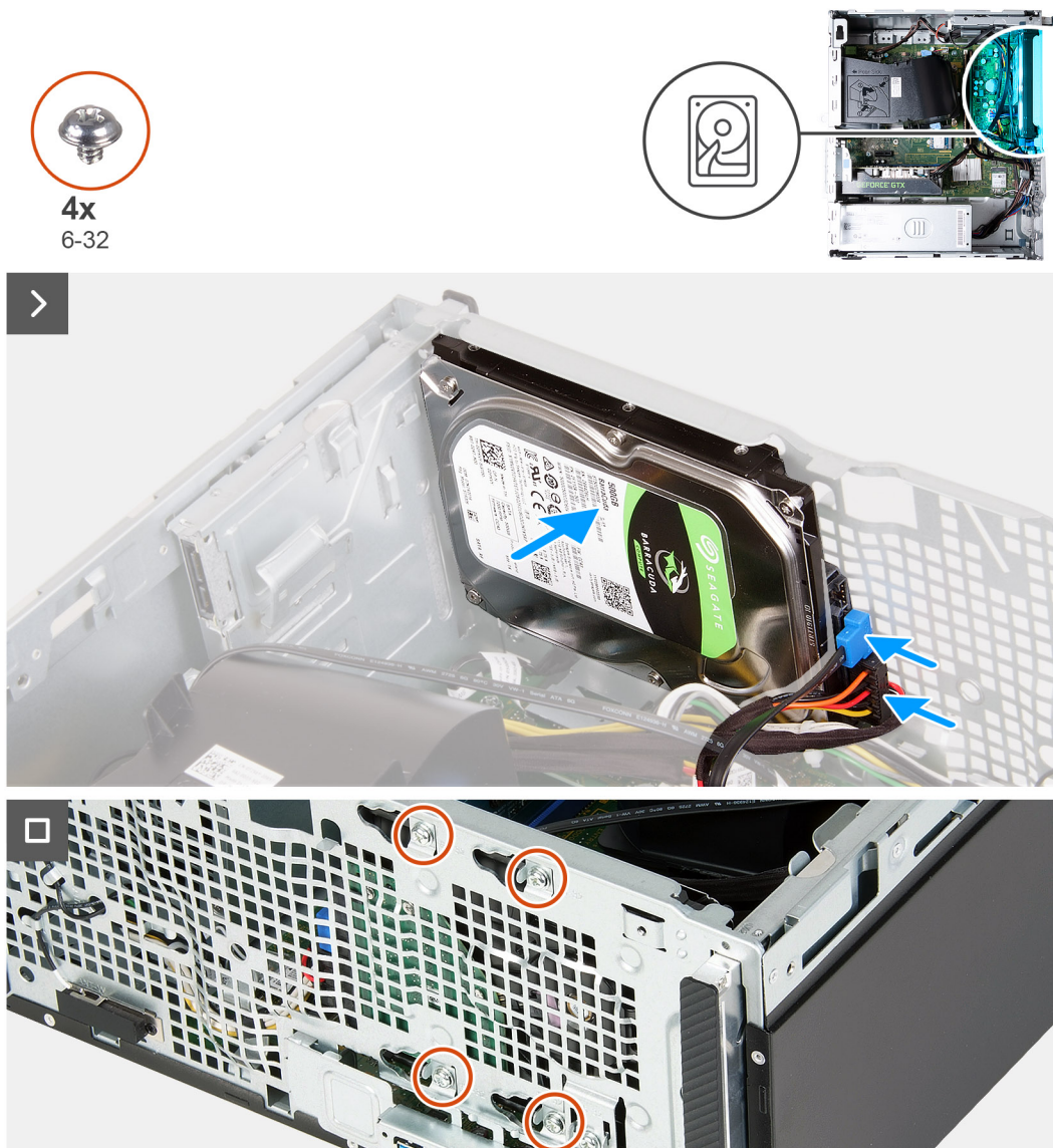
Figure 25. Installing the hard drive
