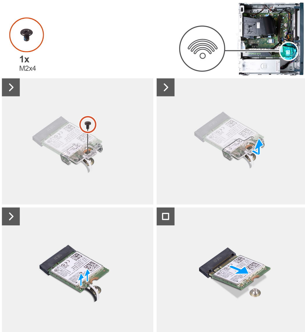
Figure 20. Removing the wireless card
