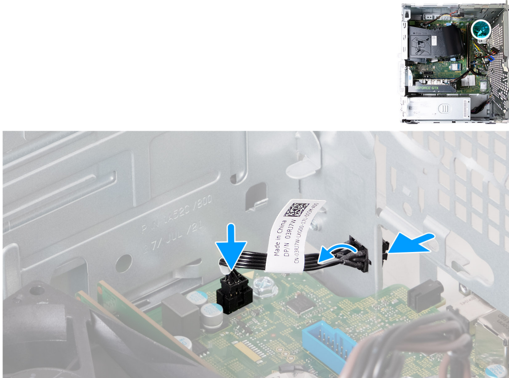
Figure 27. Installing the power button
